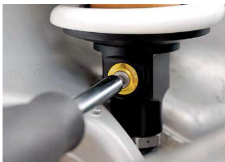
The rebound damping can be adjusted on all shock absorbers from Touratech Suspension.
